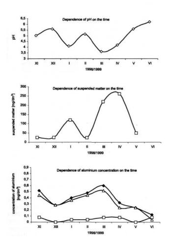
Fig. 2. Dependences of variables (pH, suspended matter,  $\diamond$  cAl<sub>tm</sub>/ $\Box$  cAl<sub>nl</sub>/ $\Delta$  cAl<sub>nm</sub> on the time) at the measuring point "Obwodnica" down from the River Silnica.
